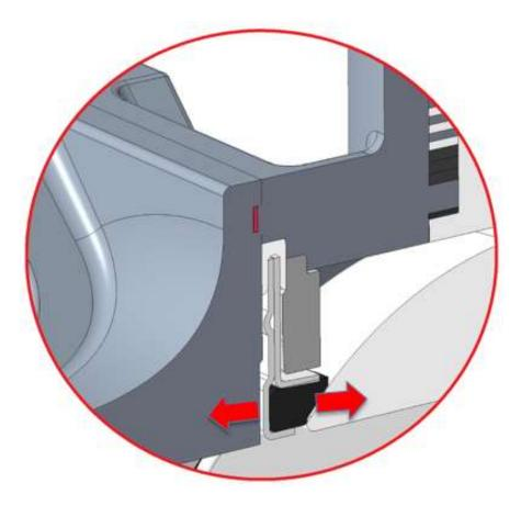
The absorption area of the medium pressure is not limited to the ball area, but encompasses the entire sealing element. In the event of an increase of differential pressure, the additional forces increase as well – the **preloaded** diaphragm springs which press against the ball are subsequently relieved and service live further improved.
